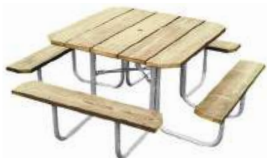
358-PT48 4-Seat 48" Square Table, pressure treated planks, galvanized frame
